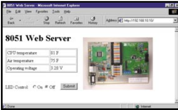
Photo 2 —Seeing is believing! The web page and image served by the 8051 can be seen in the browser window. The on/off buttons control the state of an LED on the breadboard.
